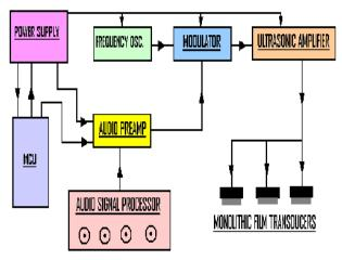
Fig3: Block diagram of a Private audio wave system
